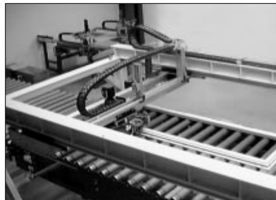
Partner for the plastics industry Automatic screwing device for window fittings with WIESEL™ SPEEDLine ®.
